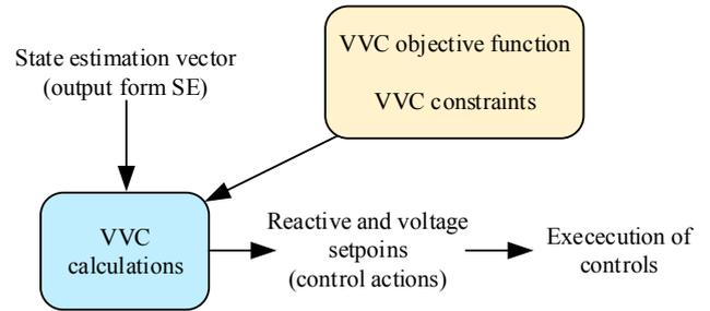
Fig. 11. VVC Flow diagram
