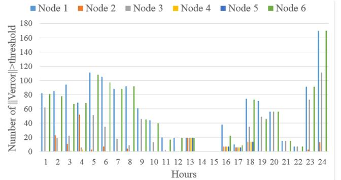
Fig. 5. Number of  $\|\vec{V}^{error}\|_2$  norm threshold exceeded during day for 6 400 kV nodes
