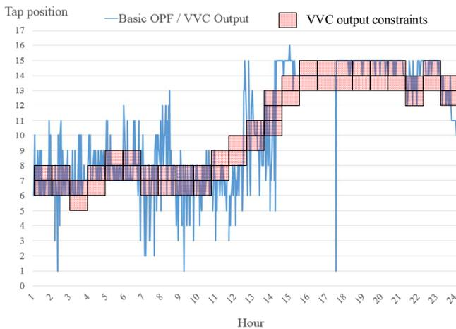
Fig. 12. VVC / OPF output for tap changer position and VVC output constraints
