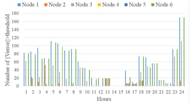
Fig. 5. Number of  $\|\vec{V}^{\text{error}}\|_2$  norm threshold exceeded during day for 6 400 kV nodes
