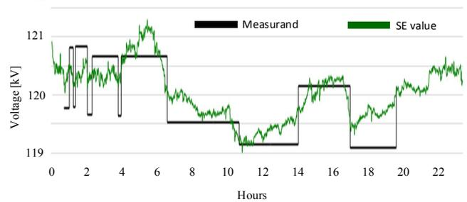
Fig. 8. Example of inaccurate SE tap changer characteristic
