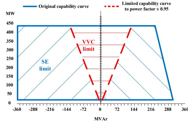
Fig. 13. Original (SE) and limited (VVC) capability curve of generator
