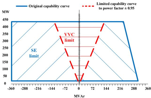
Fig. 13. Original (SE) and limited (VVC) capability curve of generator
