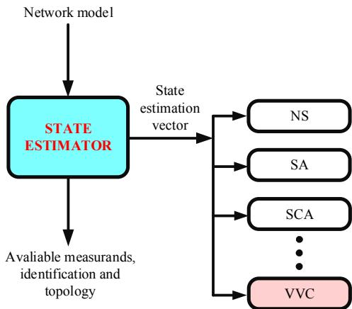
Fig. 1. Flow diagram of EMS functions
