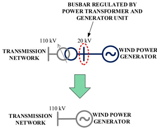
Fig. 9. Connection of wind power plant to the transmission network: with power transformer and directly, without power transformer
