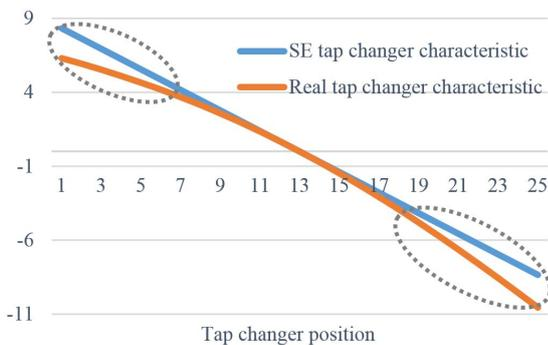
Fig. 7. Example of inaccurate SE tap changer characteristic
