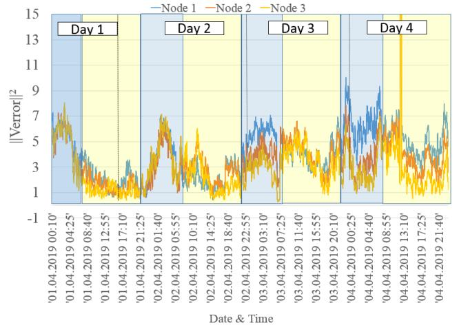
Fig. 4. Variation of the voltage error norm during four days period for three different nodes
