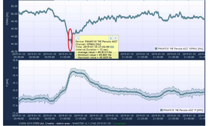
Fig. 5. f and P trends for generator 2 in Hydro PP Peruca with active frequency primary regulation in period 20:45-21:45 with marked detail in 21:02.
