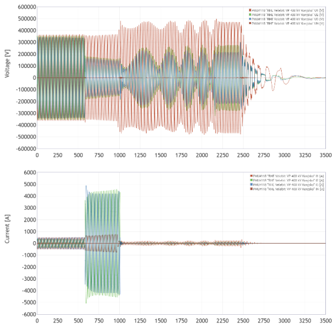
Fig. 7. All three phase voltages and currents recorded in substation Velebit for line 400 kV Konjsko, during busbar faults in substation Velebit
